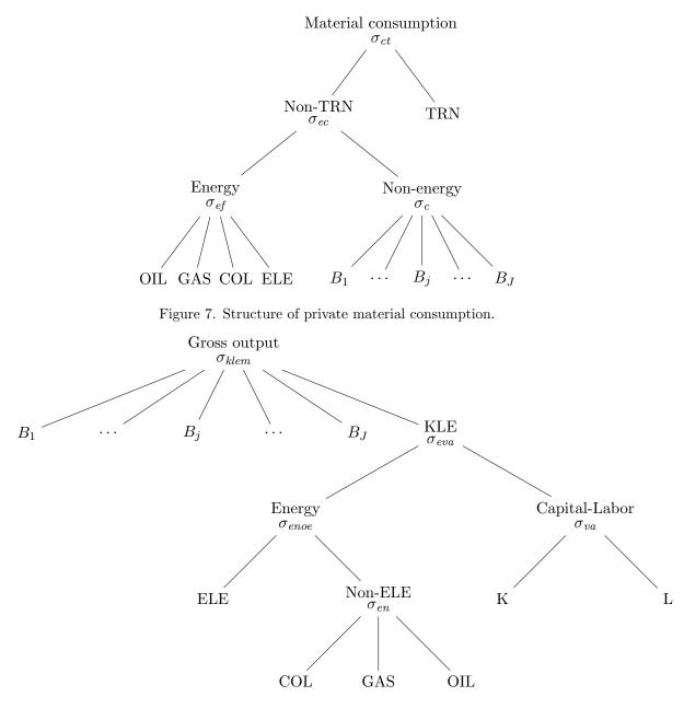
Figure 8. Production structure for final goods non-energy sectors  $g \in G = \{AGR, EIS, TRN, SRV, MAN\}$  and refining of crude oil  $c \in C = \{OIL\}$ .
