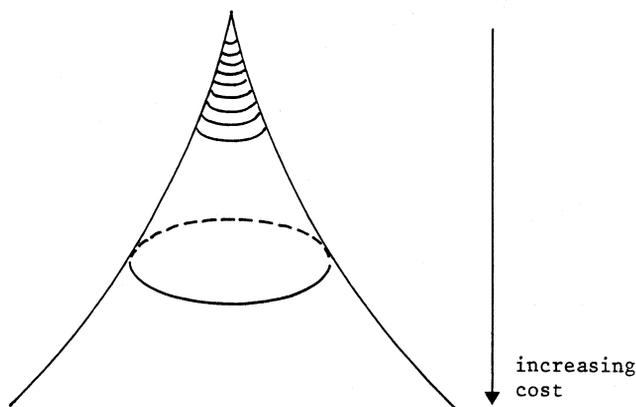
Quantity is represented by the volume of the cone, and cost increases downwards along the axis. The black top of the cone has been "cut off" by extraction until now. The remaining global economic reserves are represented by the rest of the volume above the indicated cut-off, which is determined by the market prices of the resource.
